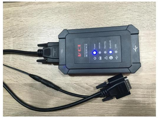
Step 1. Connect your VCI with the main cable and the 12V power as follows:
